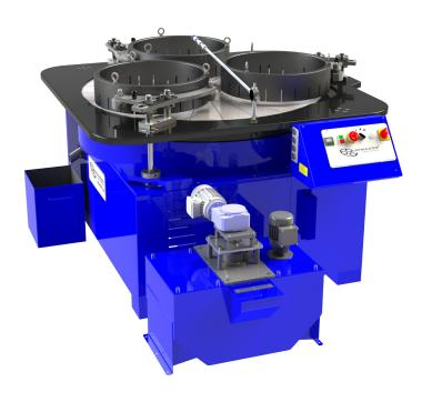
The Lapmaster Wolters model 56 is equipped with a 1422mm diameter lap plate. This is manufactured from Grade 300 grey cast iron to ISO 185(2005). It consists of individual segments bolted to a support plate.
